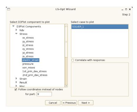
Figure 20-17 For metal forming specify that the coordinates instead of the nodes must be followed and specify the part (blank) for which the results must be mapped.
