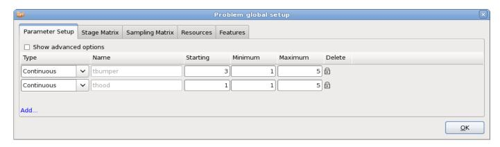
Figure 2-7: Parameter Setup dialog. Define the parameter type and required values.
