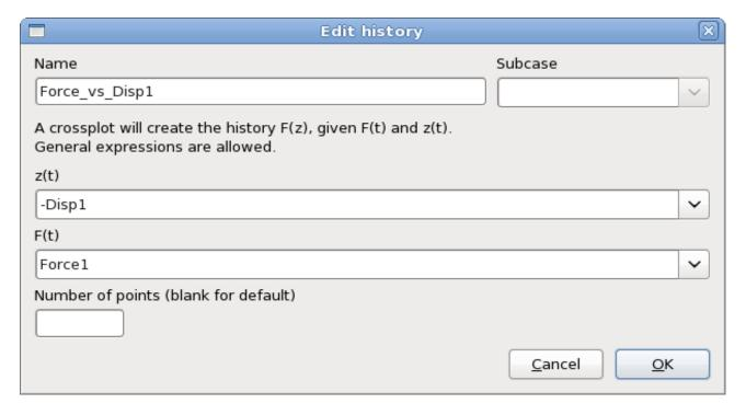
Figure 19-3: Crossplot definition of force vs. displacement
