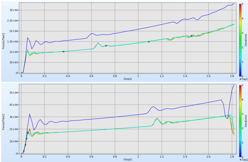
Figure 21-12: Comparison of optimal force-displacement curves and test data. The simulation curves are colored by iteration
