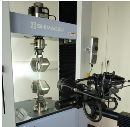
Figure 28-7: Tensile testing equipment and optical measurement system by GOM ARAMIS (courtesy Dynamore GmbH, Stuttgart).
