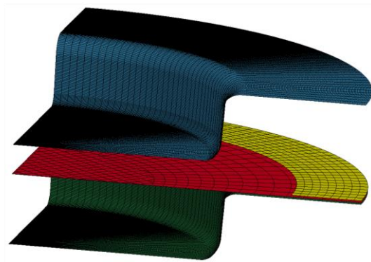
Figure 20-65: Quarter segment of FE model: tools and blank
