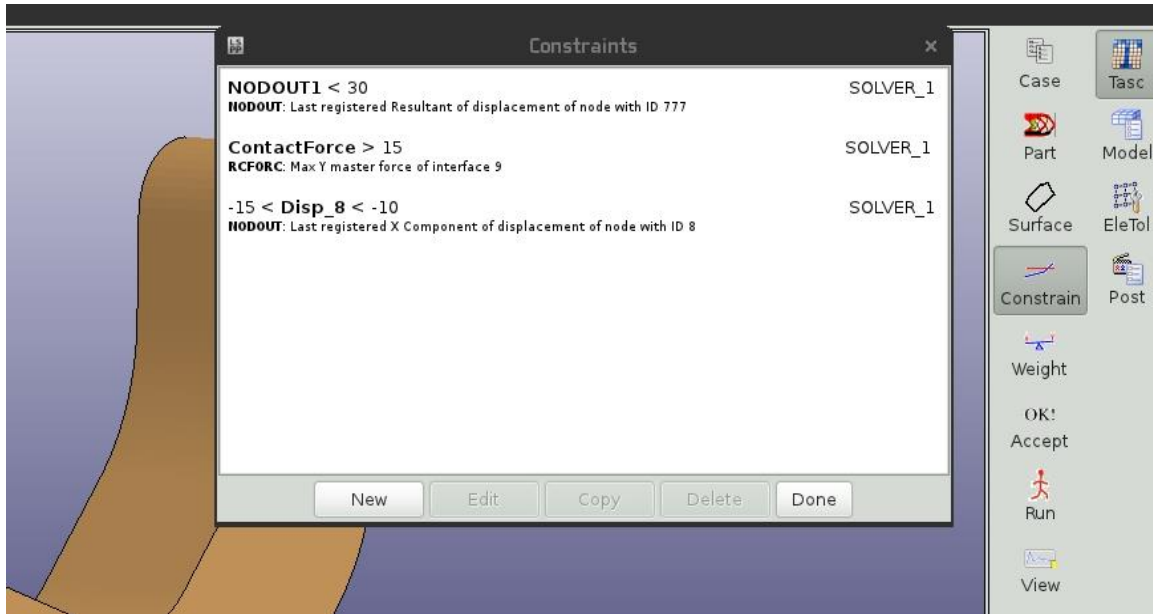
Figure 4-3: The constraints overview panel.
