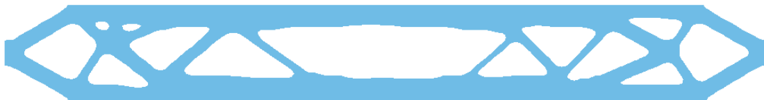
Figure 1-65: Final beam structure for MDO: iso-surface with iso-level 0.3.
