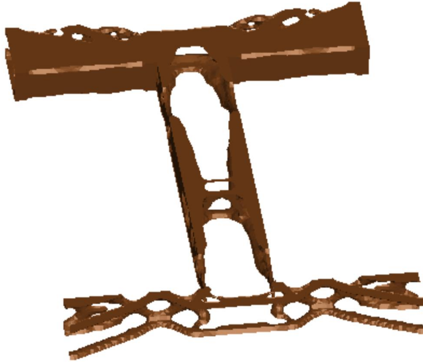
Figure 1-27: Final design for the simplified side impact problem: iso-surface with iso-level 0.5
