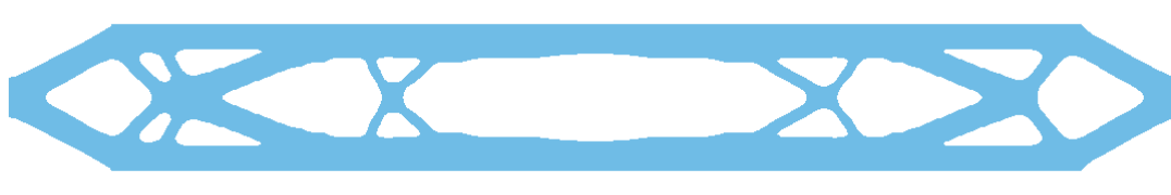
Figure 1-60: Final geometry for NVH design: iso-surface with iso-level 0.3.
