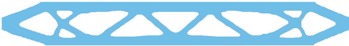
Figure 1-72: Final beam structure for MDO with multiple constraints: iso-surface with iso-level 0.3.
