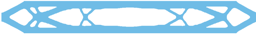
Figure 1-60: Final geometry for NVH design: iso-surface with iso-level 0.3.
