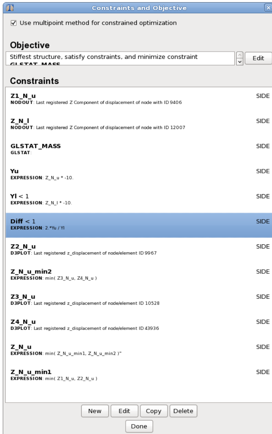
Figure 1-22: Definition of multipoint method and constraints.
