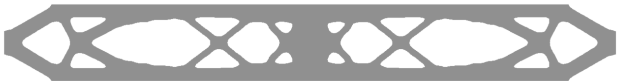
Figure 1-68: Final beam structure for NVH with a frequency constraint.
