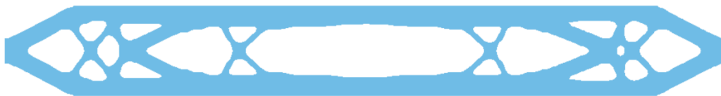
Figure 1-58: Final geometry for NVH design: iso-surface with iso-level 0.3.
