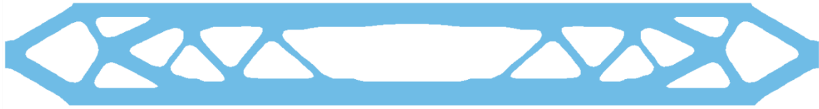
Figure 1-63: Final beam structure for MDO: iso-surface with iso-level 0.3.
