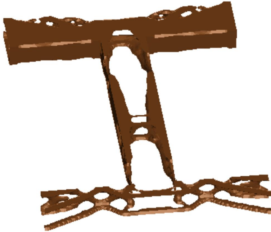
Figure 1-25: Final design for the simplified side impact problem: iso-surface with iso-level 0.5
