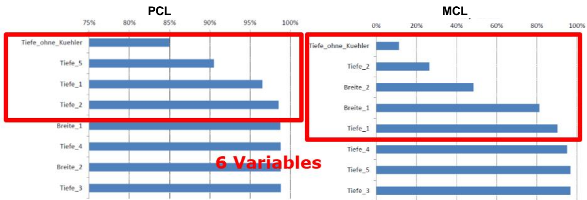
Fig.6: Cumulative Distribution of design Variables. Only 6 variables contribute significantly to the target function
